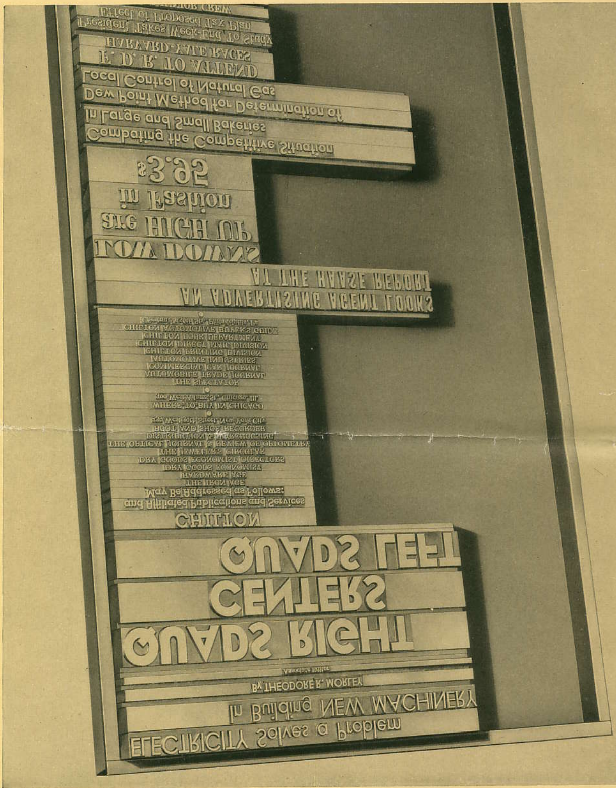
The Autospacer quads right, centers, or quads left, as required—any size of type, any width of line, and any number of characters (even a single character)—with or without the use of spacebands. Fully justified composition is set in the regular way.
